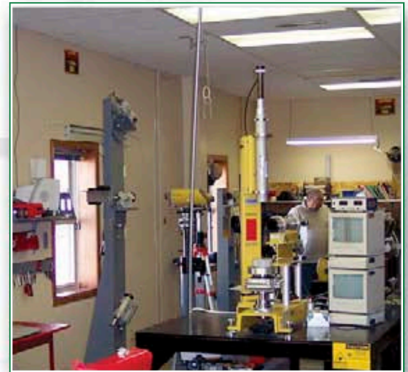
Pictured above is our Topcon Video Range used to calibrate rotating lasers with very high precision.
